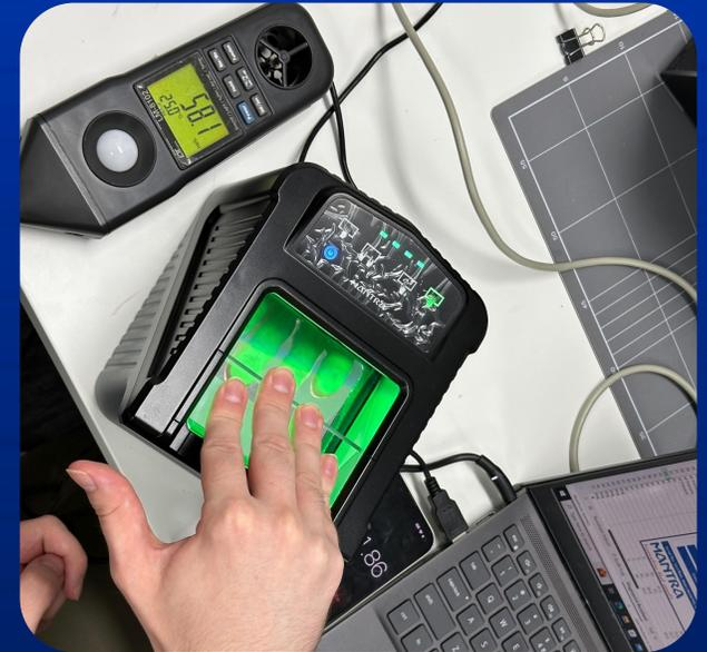
Image showcasing testing of an optical fingerprint scanner – for elevated angle test scenario
